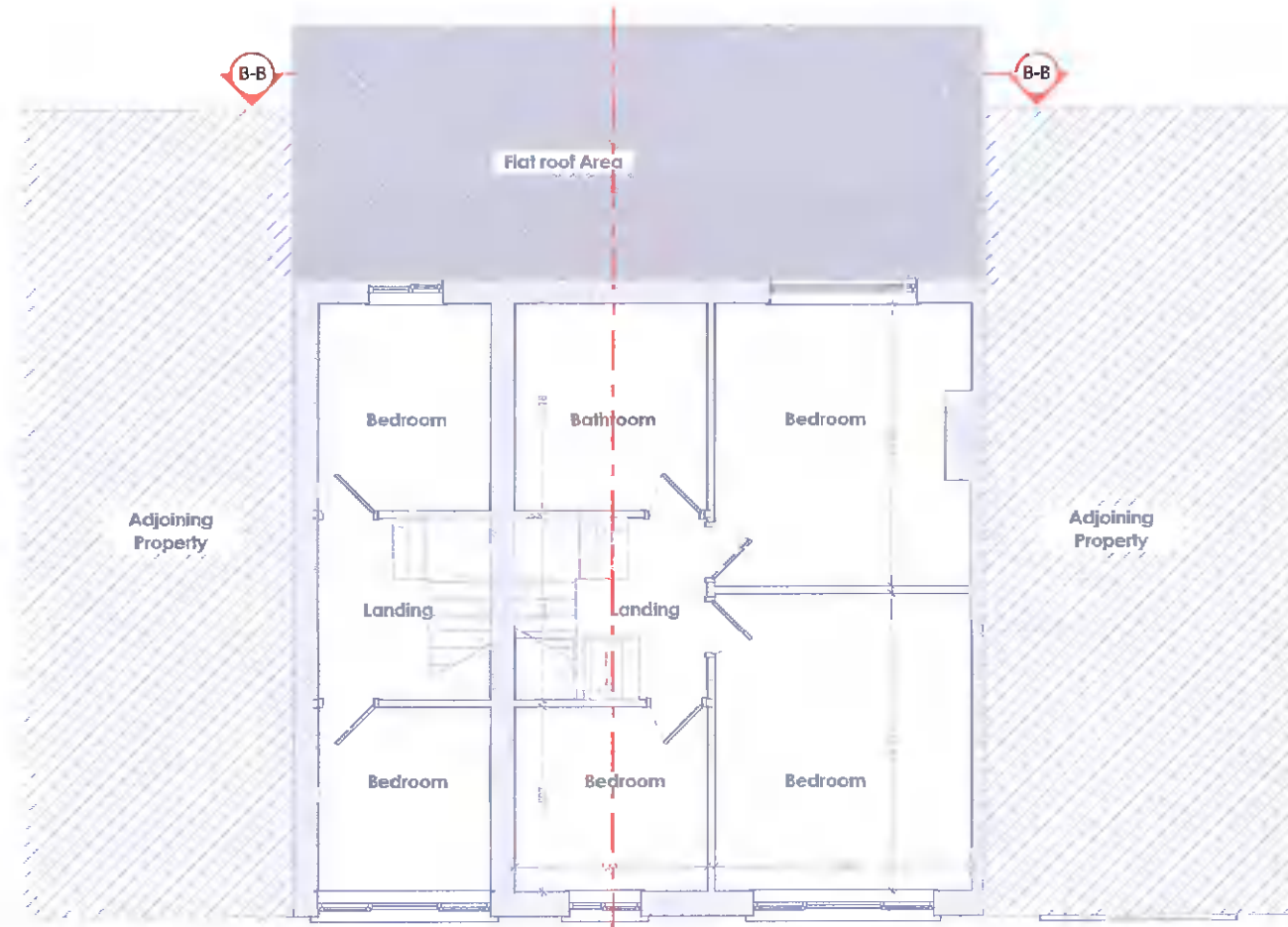
Existing Floor Area = 70.904 m 2 Existing - First Floor 1:100
