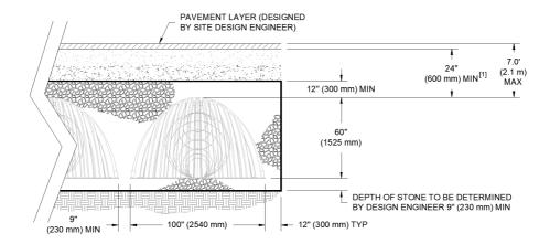
[1] - TO BOTTOM OF FLEXIBLE PAVEMENT. FOR UNPAVED INSTALLATIONS WHERE RUTTING FROM VEHICLES MAY OCCUR, INCREASE COVER TO 30" (750 mm).
