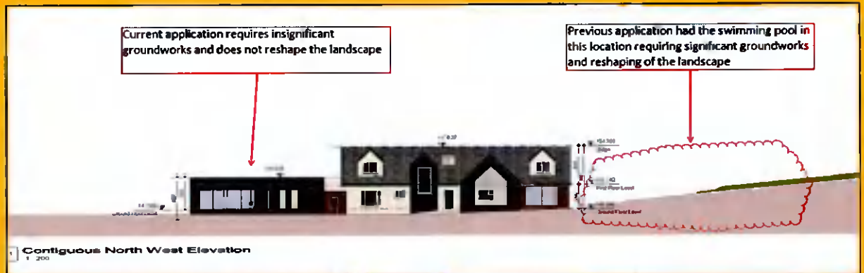
Figure 1.3: Elevation Drawing Showing Location of Development of the Previous Refusal at the Site Which Required Significant Amounts of Cut and Fill which is not Required as part of the Subject Application.
