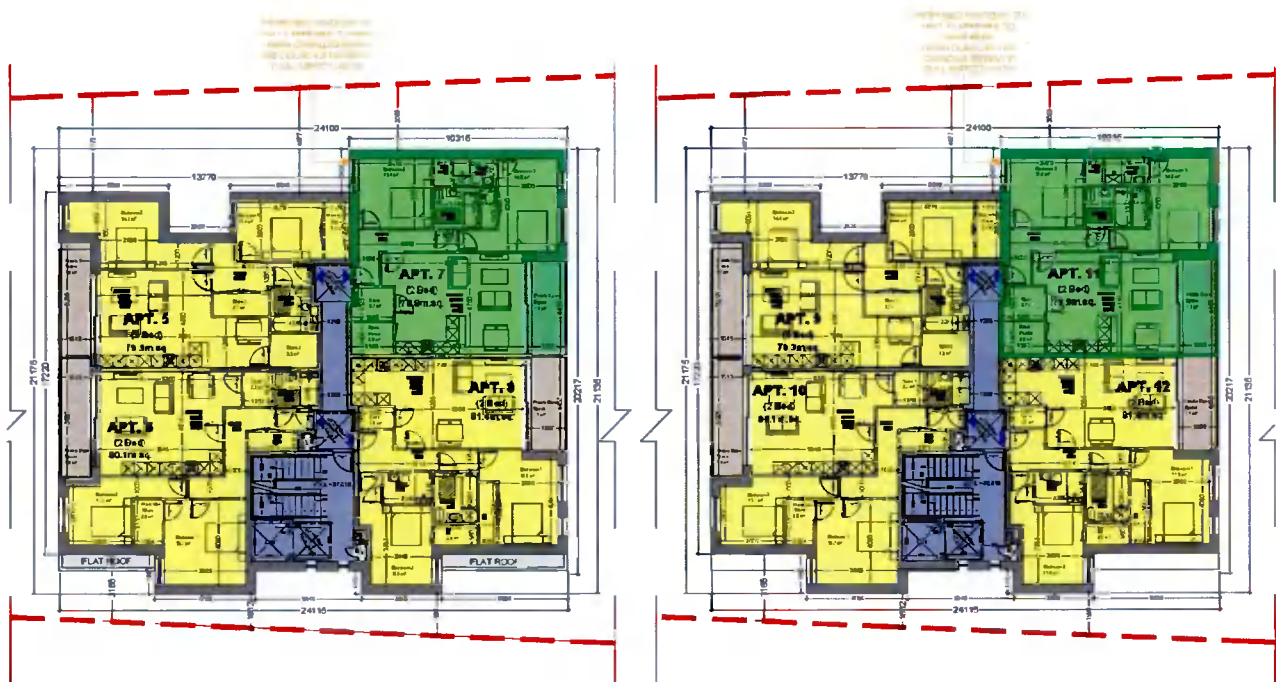
Reference Image 1: highlighting unit no 7 at first floor level (left) and unit no 11 at second floor level (right) highlighted in green which were excluded in the council's calculations of dual aspect units
