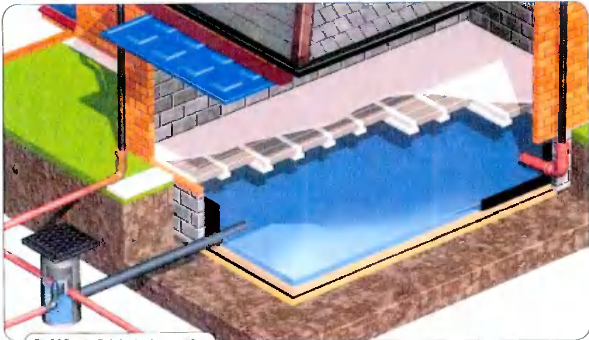
Fig. 2.6 Garastor. Typical system (garage void)
