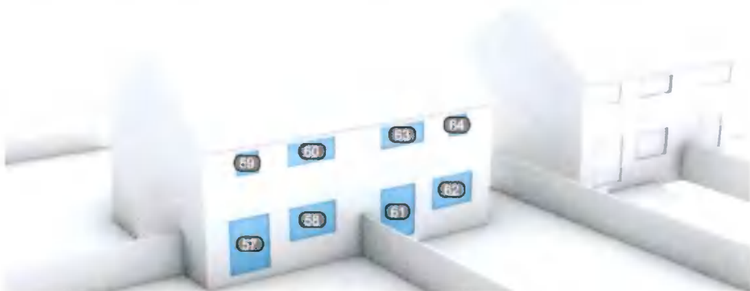
Figure 13: View of model of No.s 170 & 172 Kennelsfort Road Upper, locating of windows assessed for VSC.
