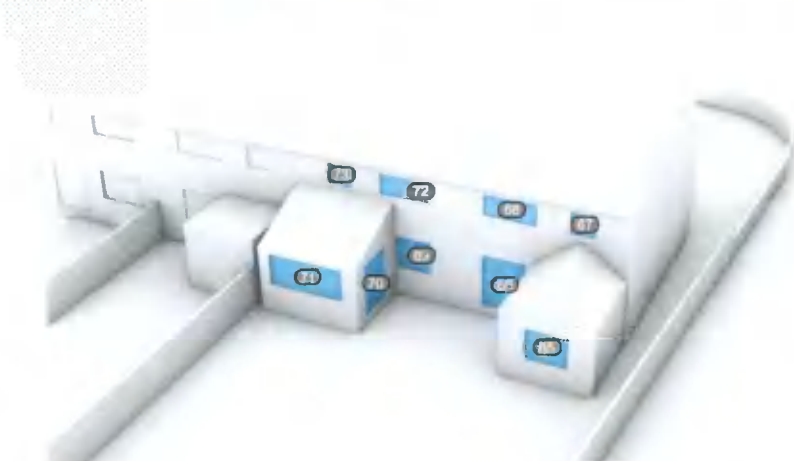
Figure 15: View of model of No.s 215 & 215A Palmerstown Ave, locating of windows assessed for VSC & APSH.
