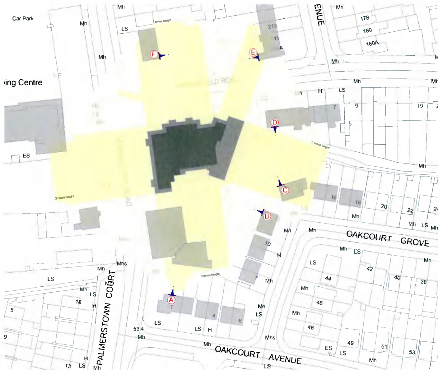
Figure 2: Proposed site plan showing the zone of influence and the direction of window walls in adjacent residential properties.
