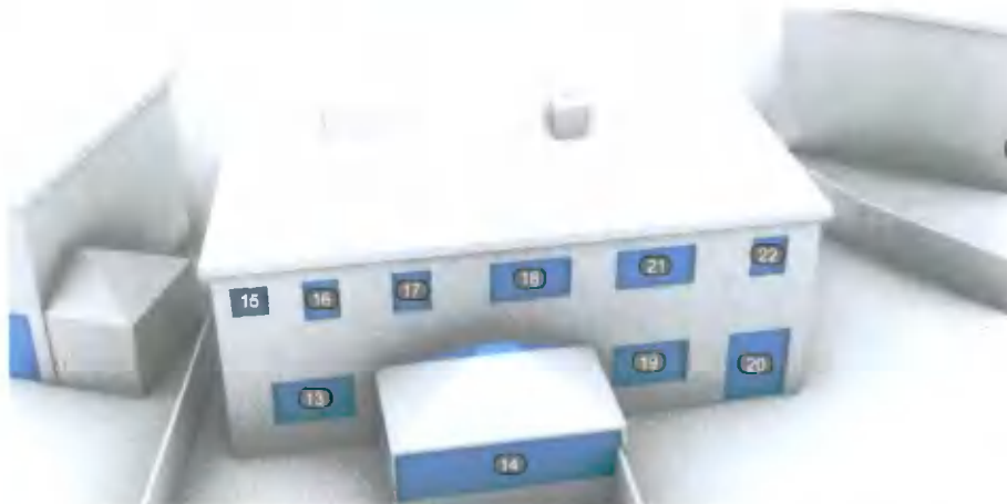
Figure 7: View of model of No.s 13 & 14 Oakcourt Grove, locating of windows assessed for VSC.
