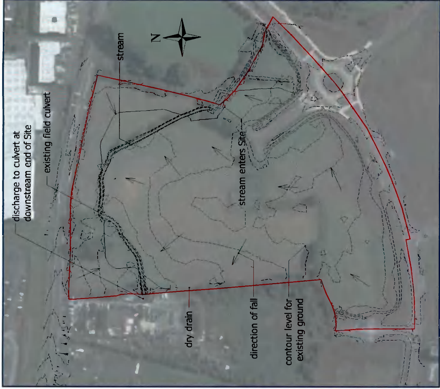
Figure 3-2 Site Topography / Main Drainage Features
