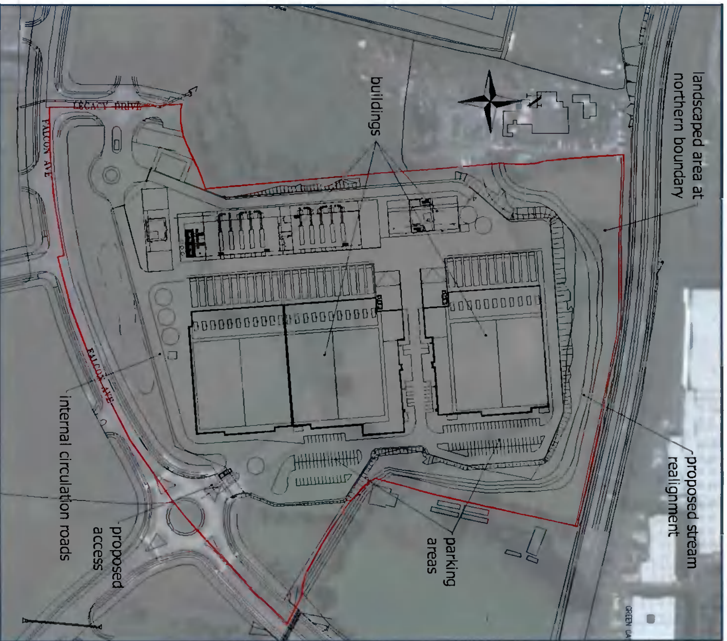
Figure 4-1 Schematic Layout of Proposed Development
