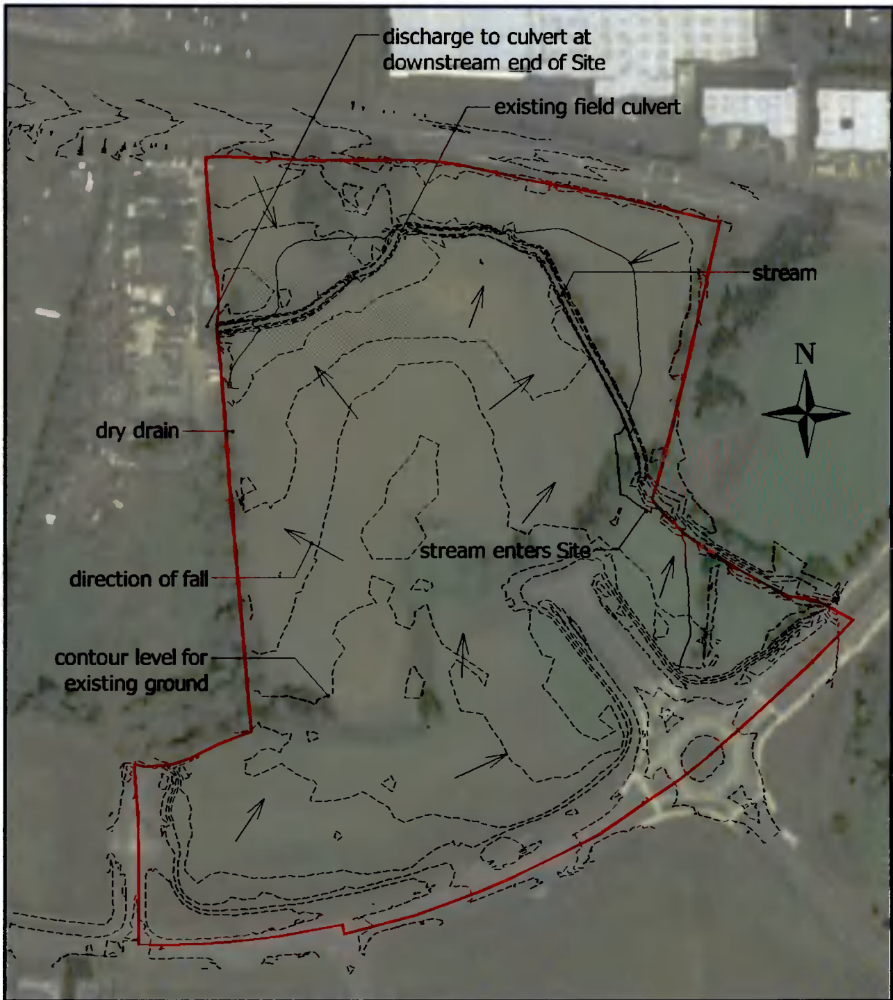
Figure 3-2 Site Topography / Main Drainage Features
