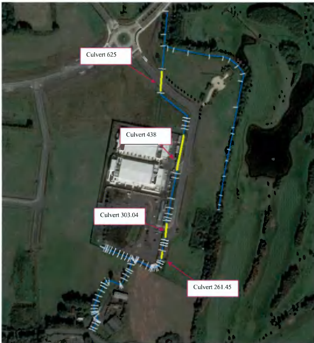
Figure 23: Culverts location – aerial view
