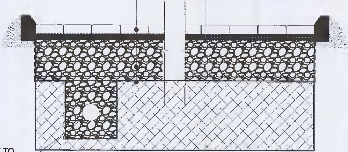
HYDROPAVE CONSTRUCTION DETAIL SCALE 1:20
