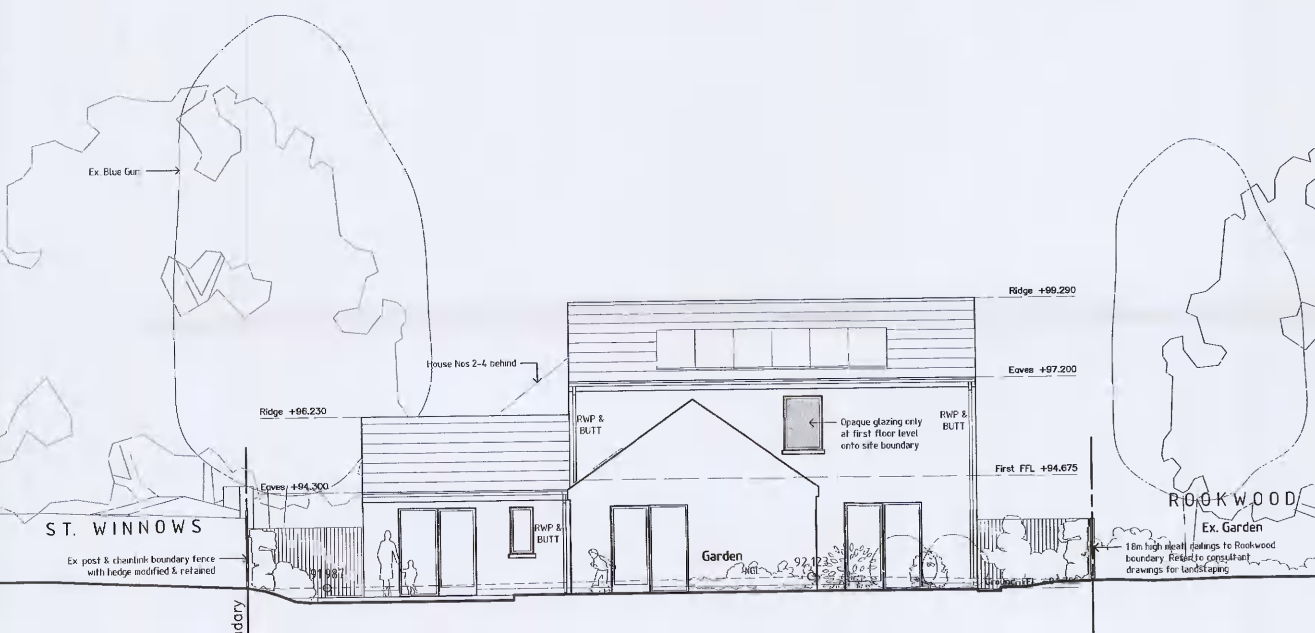
SOUTH-EAST ELEVATION (to adjoining SHD)
