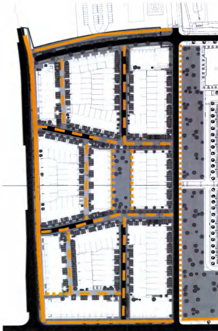
Figure 5-2 - Aderrig Phase 2 Cyclist Provision
