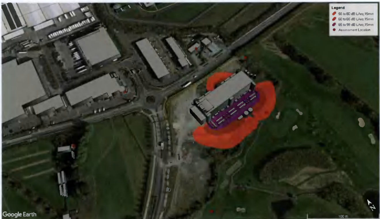
Figure 7 Generator Testing Noise Contour (Scenario C) – Extent of 55dB(A) Contour
