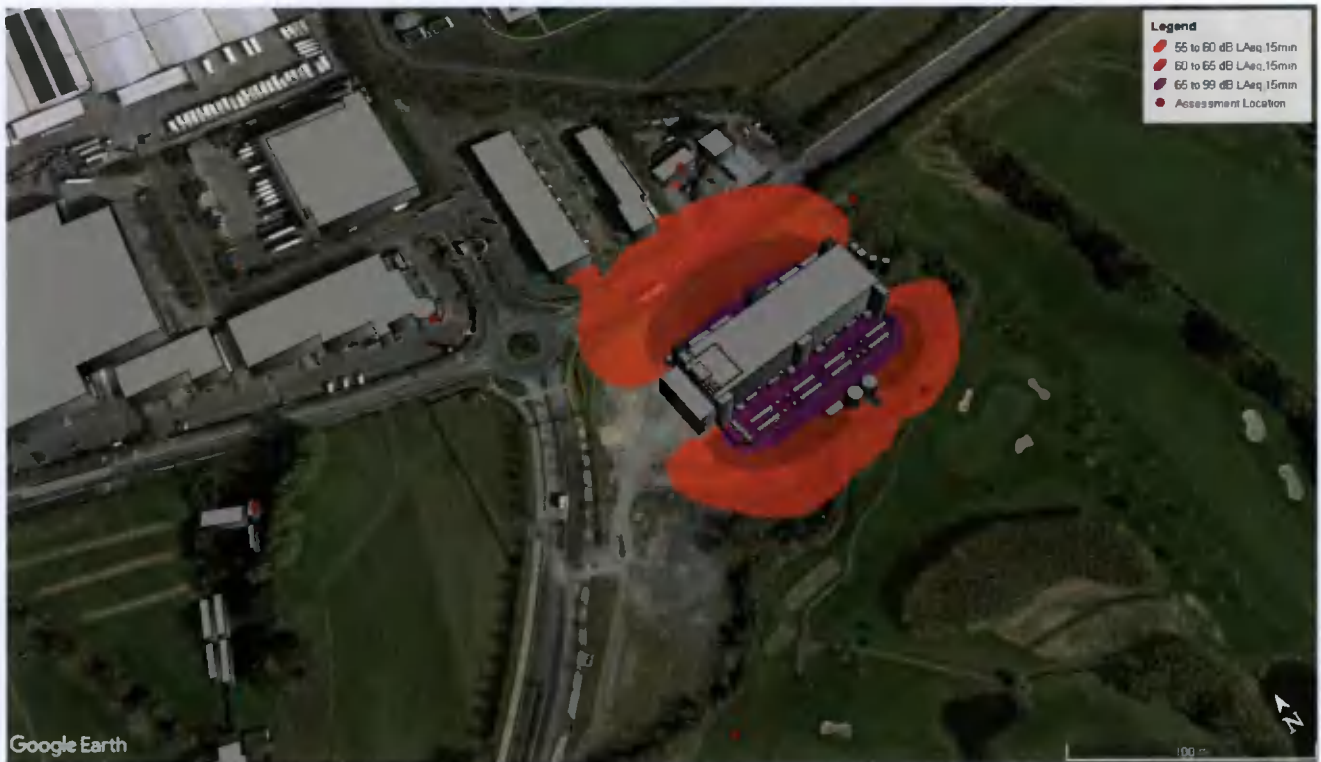
Figure 6 Emergency Operations Noise Contour (Scenario B) – Extent of 55dB(A) Contour
