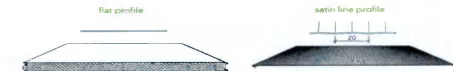
Picture 42: Composite cladding textures: flat for the proposed building, satin line (also called micro ribbed) for the generators enclosure.
