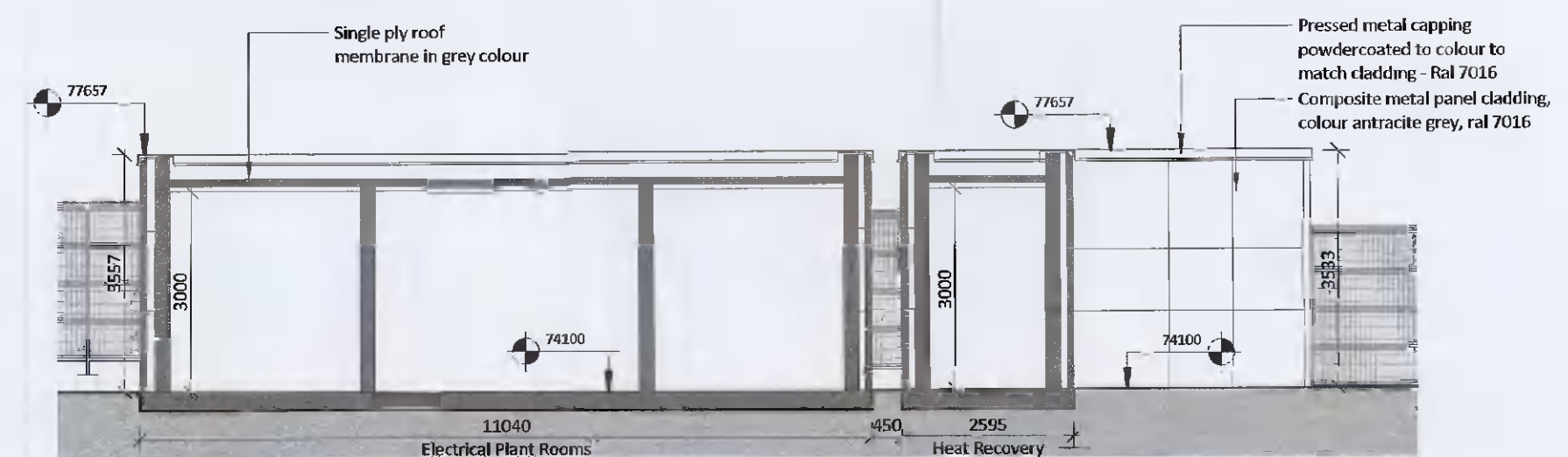
3 Heat Recovery/Electrical Plant Room Section 1 : 100
