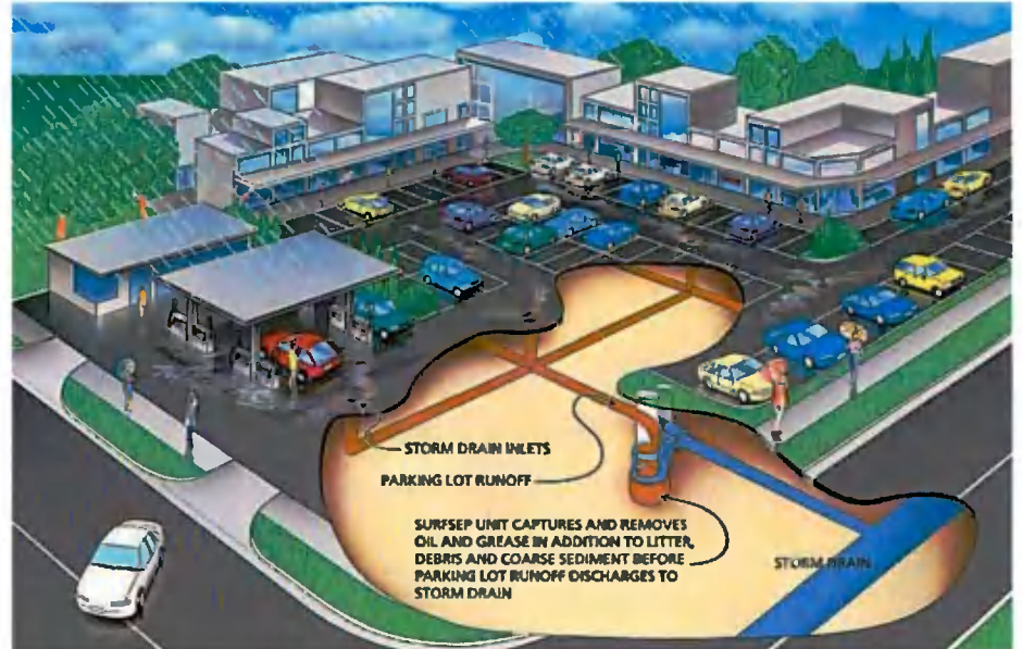
Typical SurfSep installation
