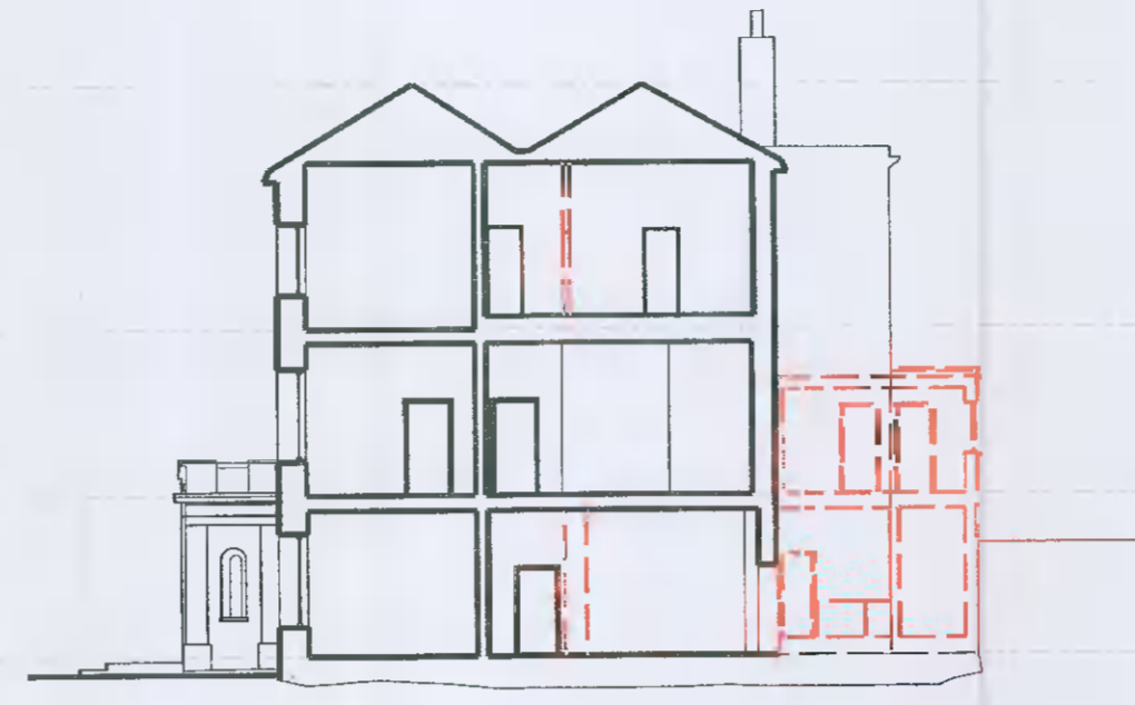
DEMOLITION - SECTION A-A 1:200 NOTE - DOTTED RED LINE INDICATES ELEMENTS PROPOSED FOR REMOVAL OR AMENDMENT
