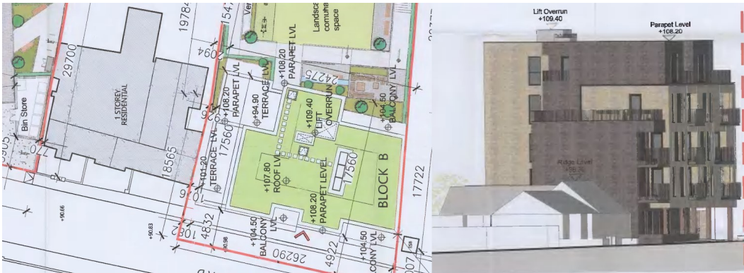
FIG. 42: THE SETBACKS TO NO. 8 ARE INSUFFICIENT
