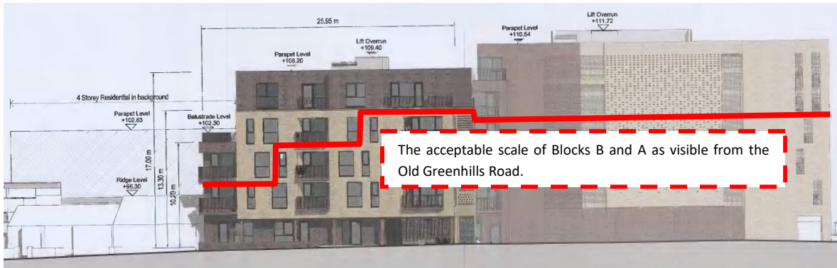
FIG. 38: BLOCK B NEEDS TO BE REDUCED TO 2, 3 & 4 STOREYS ADJOINING A 3 OR 4 STOREY BLOCK A
