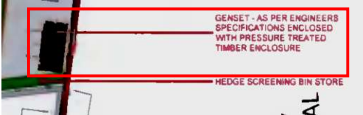
FIG. 72: PROPOSED BACK UP GENERATOR PROPOSED TO ADJOIN NO. 10 – COURT COTTAGE – OLD GREENHILLS ROAD
