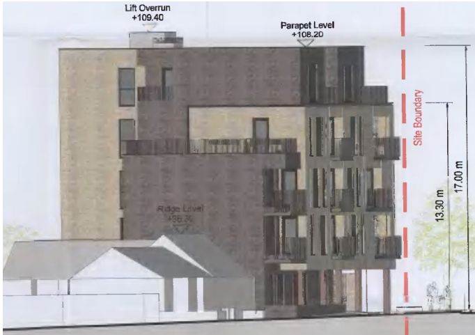
FIG. 43B: THE SITING, HEIGHT, SCALE, BULK AND DESIGN OF BLOCK B RELATIVE TO NOS. 8, 9 & 10
