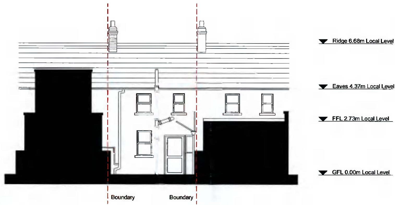
2 EX04 EXISTING: EAST (REAR) ELEVATION
