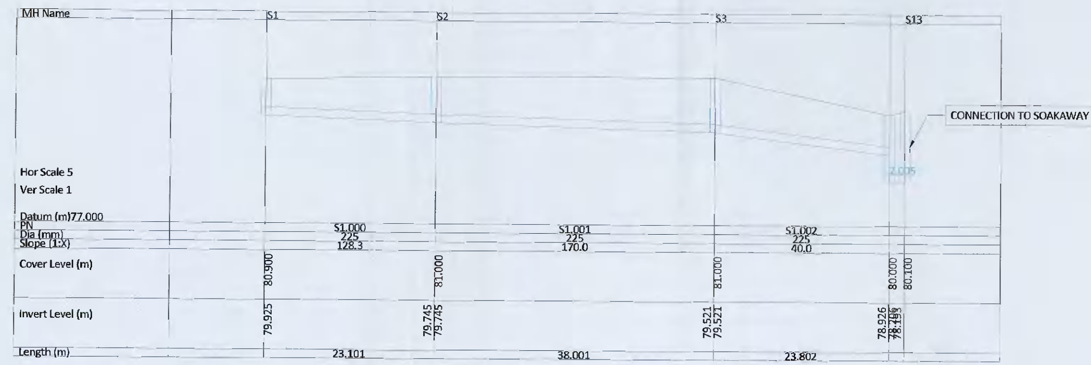
SURFACE WATER NETWORK S1.000 - S1.003
