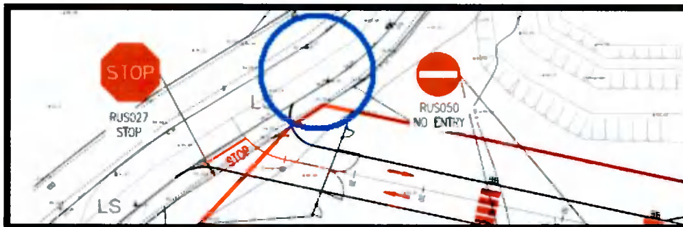
Figure 10 – No facilities for pedestrians and cyclists to cross the access road to the school entrance.
