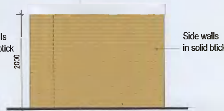
5 Substation Side Elevation Scale 1:50
