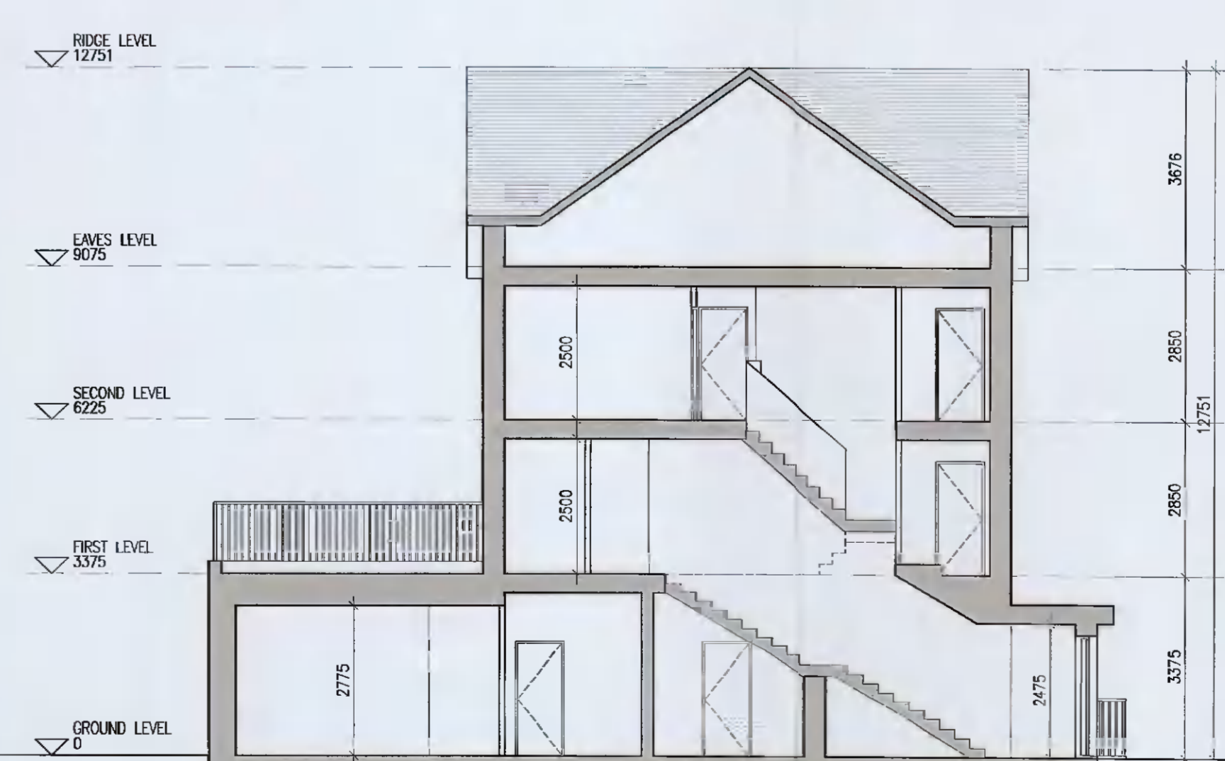
08 Typical Section [A-A] P-211 1:100@A1
