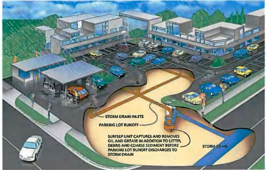
Typical SurfSep installation
