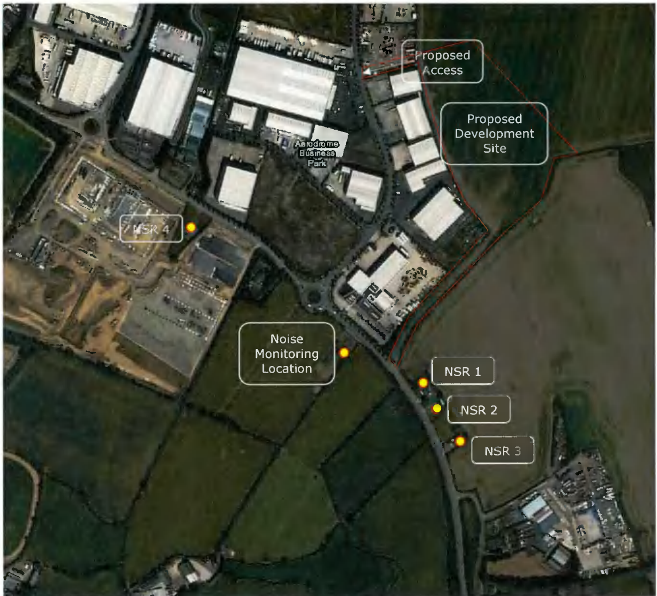
Figure 1: Step 1 – Noise monitoring location and noise sensitive receiver locations entered into noise prediction model.
