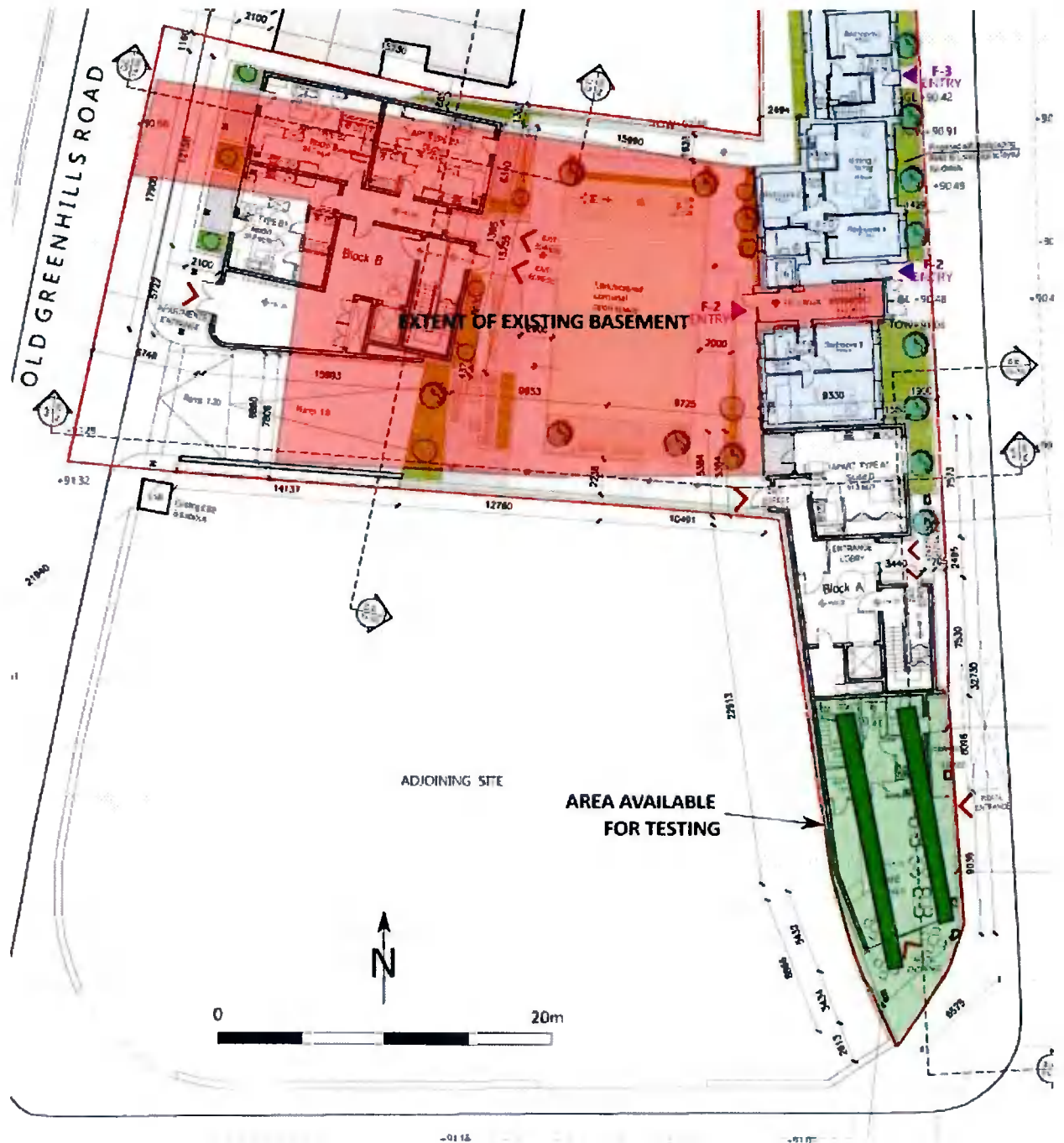
Fig. 3 detail of proposed ground floor plan showing extent of existing basement area of new retail unit extension to the south – with proposed test trench layout.
