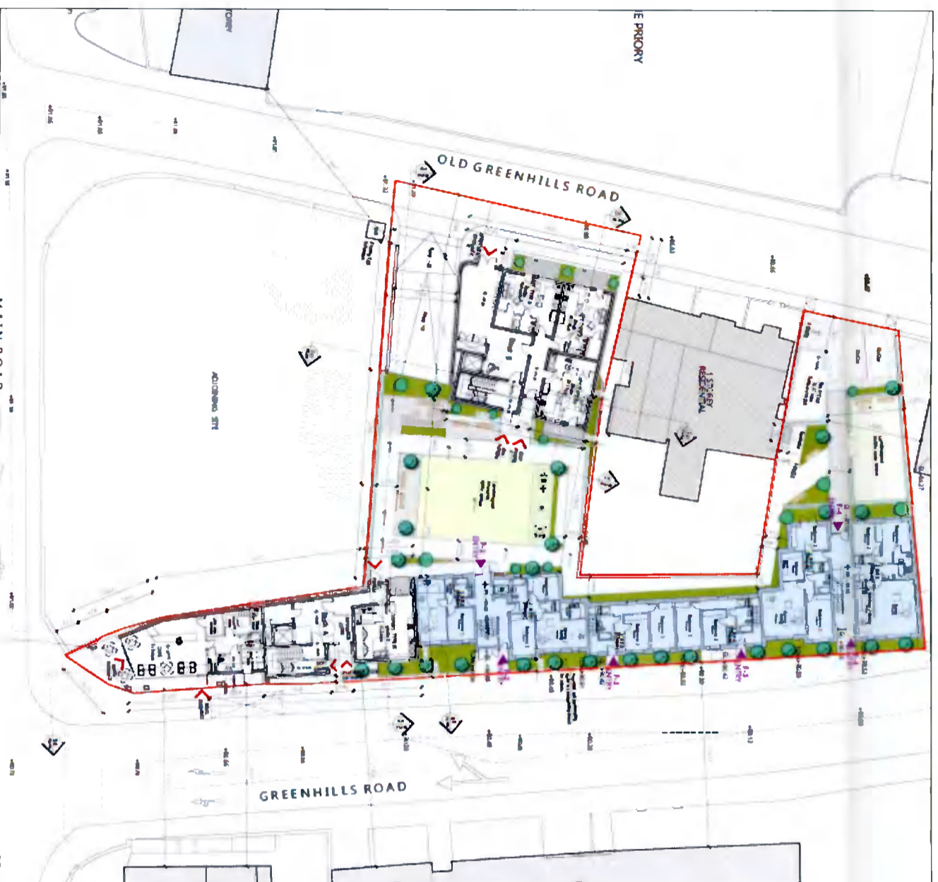
Figure 4.3 Extract of the Proposed Ground Floor Plan (Drawing No. 19118_PA-207) which shows the proposed landscaping and minimum separation distances from nearby neighbouring properties. (source: TOT Architects, cropped by Tom Phillips + Associates, 2021.)
