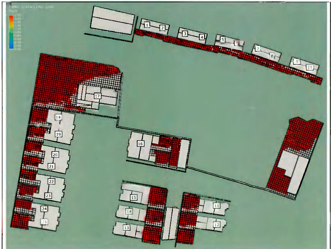
Current Scenario – March 21 st Cells coloured red if they receive \geq 2 hours of sunlight
