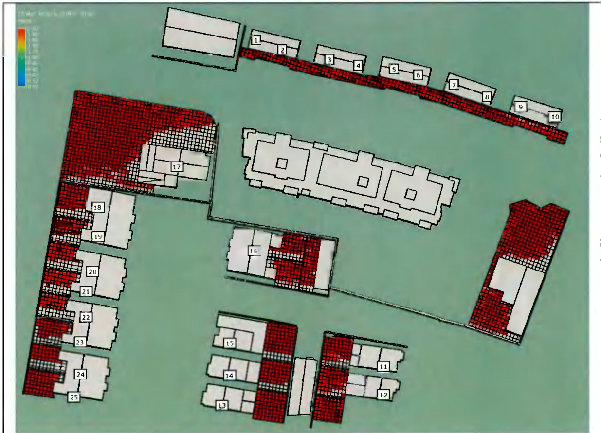
Proposed Scenario – March 21 st Cells coloured red if they receive \geq 2 hours of sunlight
