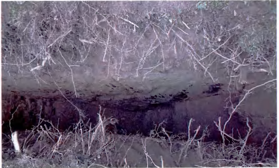
Trial Pit – Depth 2.0m – no watertable
