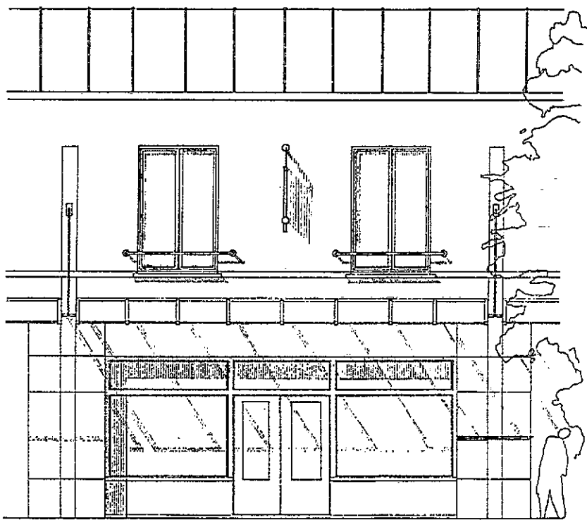
SHOP FRONT ELEVATION & PART SECTION WITH HANGING SIGN
