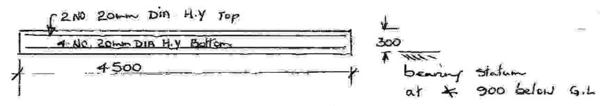
1: 50 Elevation of 900mm wide footing Min wer to reinforcing of 50 mm.
